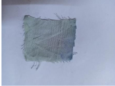
Figure 3.2 – Rubbing at wet condition at 25 cycles
