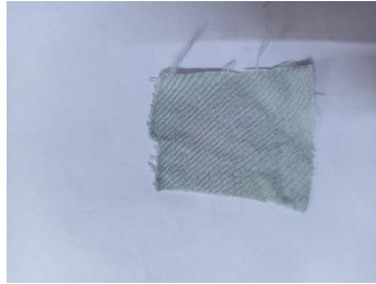
Figure 3.3 – Rubbing at Dry condition at 25 cycles
