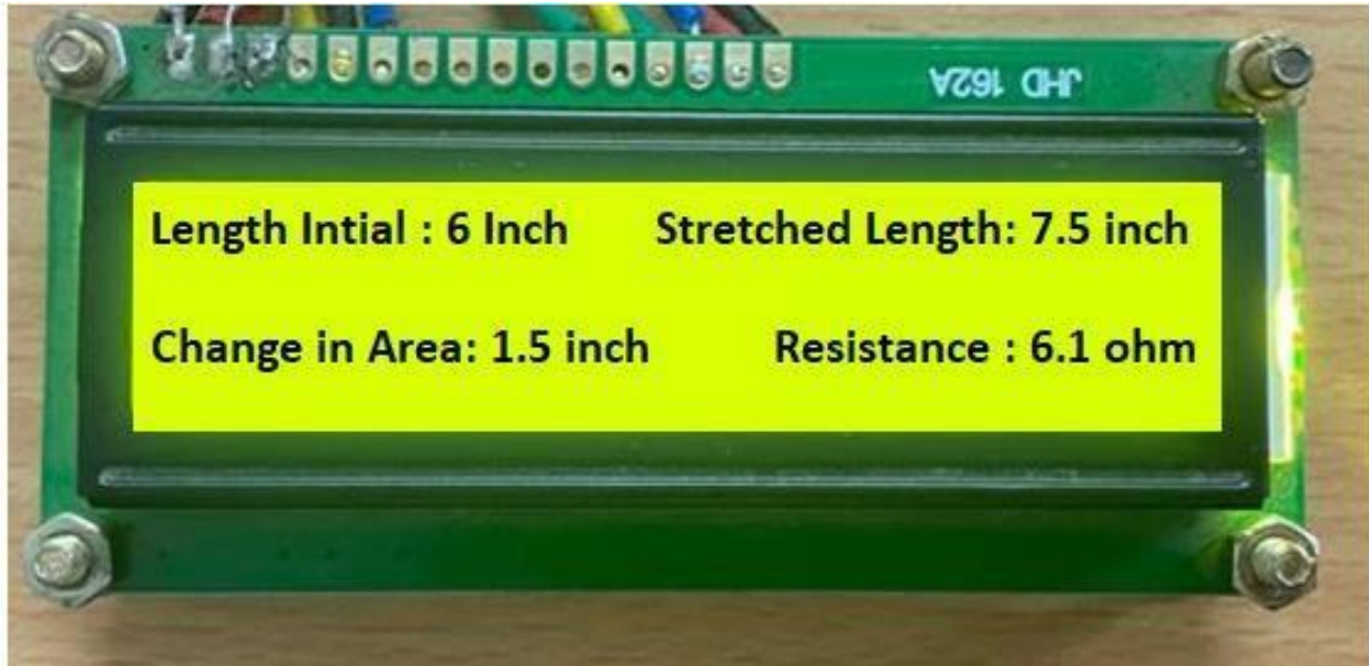
Figure-5: Digital display to show the sensor output
