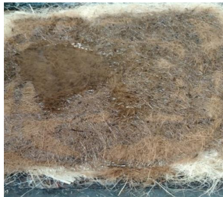
Figure 1.8 Pouring of epoxy resin and hardener mix to the fabric
