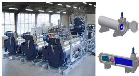
Fig.1 Commercial supercritical carbon dioxide beam dyeing machine.
