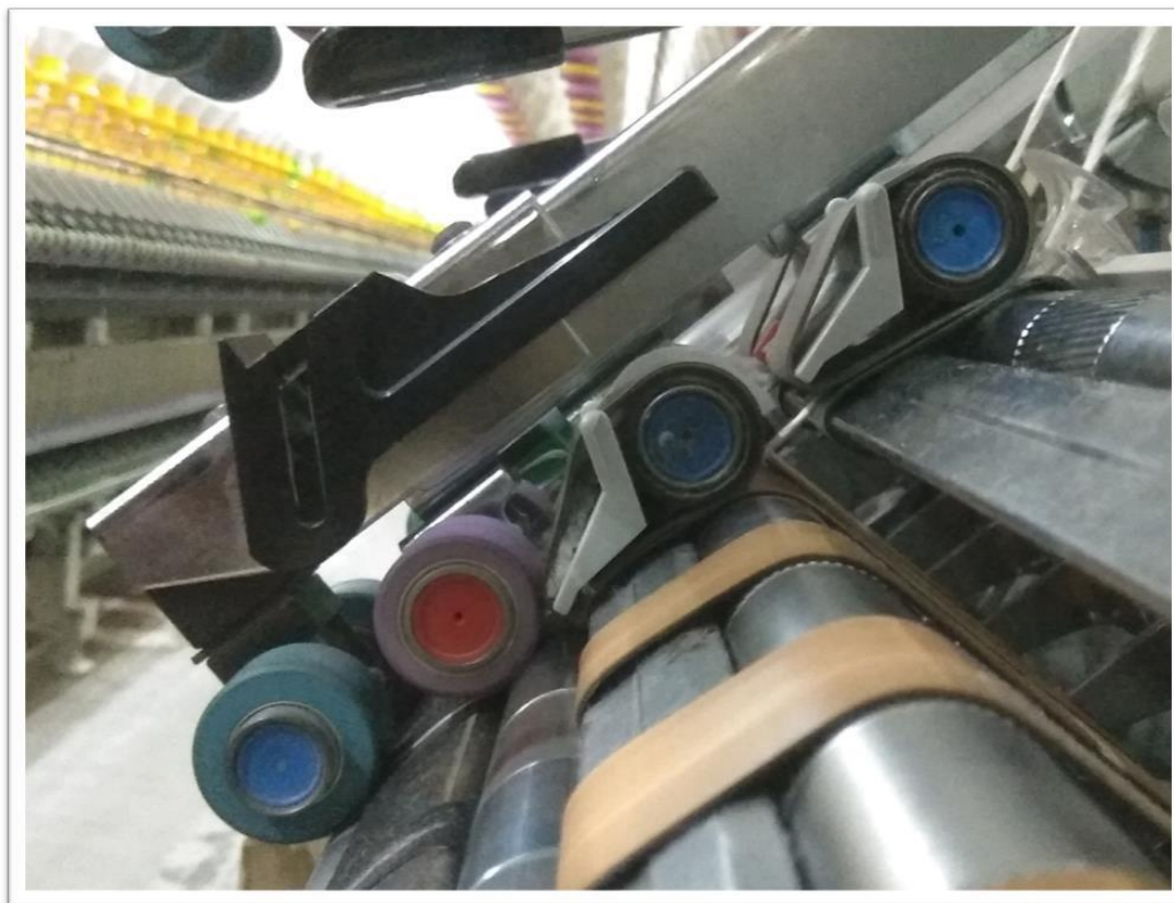
Figure -4: Machinery representation of Drafting system with Double apron guidance in compact ring frame
