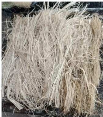
Figure 1.6 Placing abaca fibre on Board plate
