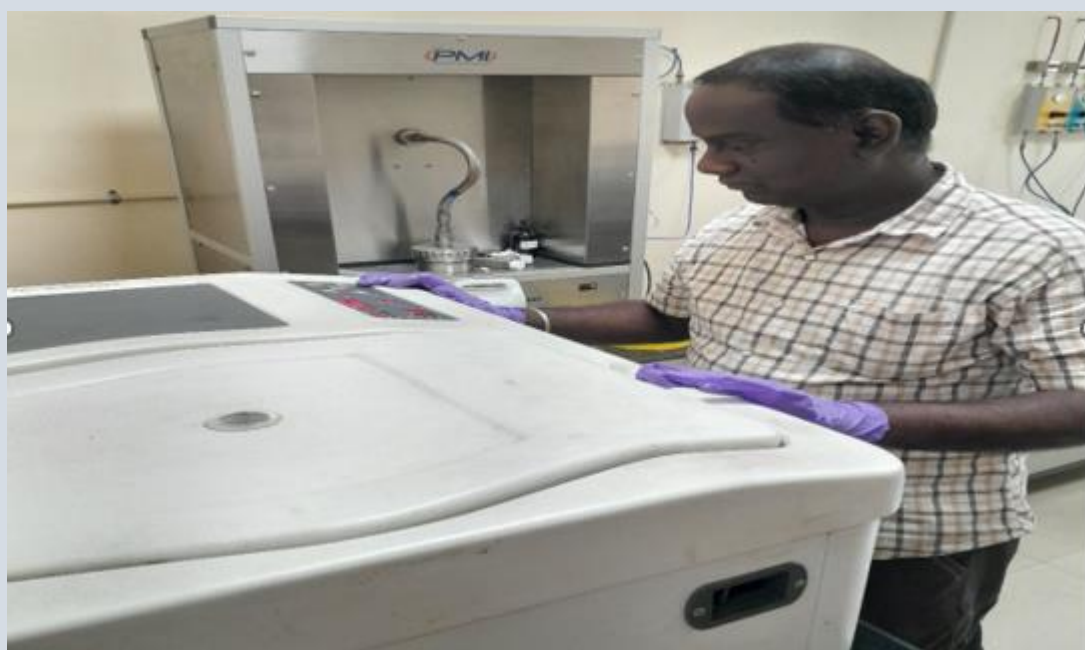
The above shot depicts the work during the preparation of ZIF-7 Nano composite in Centrifuge Machine to Settle down the Nano Particles, from the solution.
