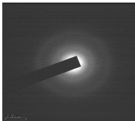
Figure 5c. HRTEM micrograph of PANI / ZnO Figure 5d. SAED pattern of PANI / ZnO
