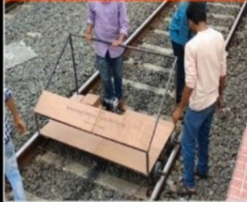
Automated Rail Monitoring for NDT Fault Detection
