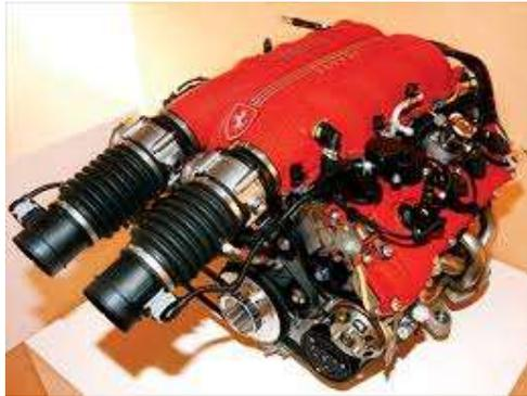
Ferrari engines are musically engineered to sound perfect by utilizing 3rd and 6th harmonics on the air intake, like an organ or flute.
